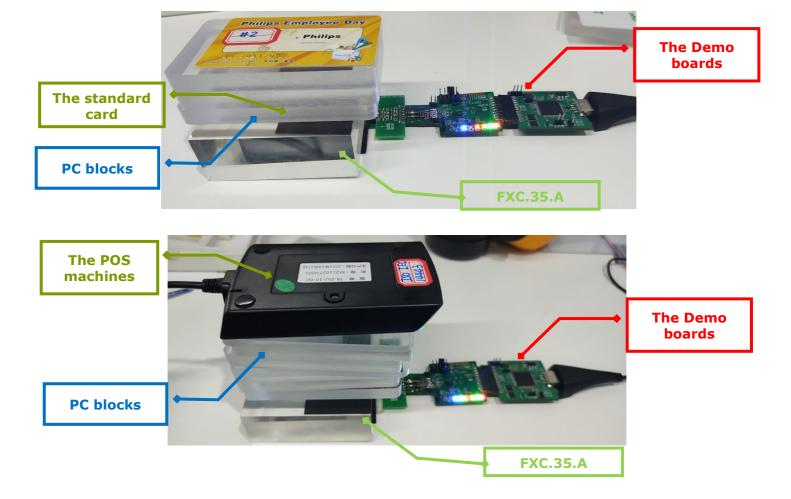
When the number of the PC material blocks are carefully adjusted until the reader can no longer read the sample, that's mean in this point the FXC.35.A cannot establish communication with the standard card or the POS machine, the thickness of the PC material block is the maximum interrogation distance of them.
