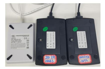
ACR122 is a PC-linked contactless smart card reader/writer developed on the 13.56MHz Contactless (RFID) Technology and followed the ISO/IEC18092 Standard for Near Field Communication (NFC), supporting not only MIFACE® ISO 14443 A and B cards but also NFC and FELICA contactless technologies.
