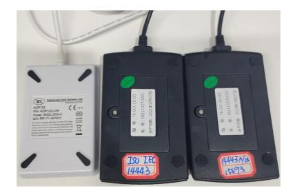
ACR122 is a PC-linked contactless smart card reader/writer developed on the 13.56MHz Contactless (RFID) Technology and followed the ISO/IEC18092 Standard for Near Field Communication (NFC), supporting not only MIFACE<sup>®</sup> ISO 14443 A and B cards but also NFC and FELICA contactless technologies.
