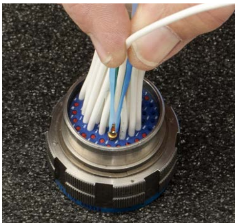
Typical All Plastic Tool Operation
