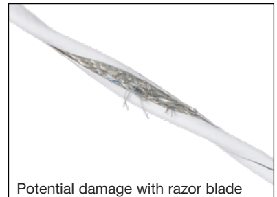
Potential damage with razor blade
