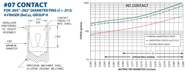
**The insertion / extraction force characteristics above** were derived using a 30 microinch gold-plated contact and polished steel gauge pins having a bullet-shaped tip. The curves represent typical average values; they are best used to compare the differences between similar size contacts and to guide you in selecting one that is suitable for your application. Your results may vary, so for your specification, we encourage you to obtain complimentary samples for your evaluation.
