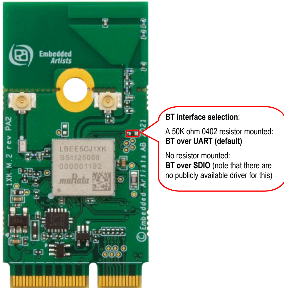
Figure 5 – 1XK M.2 Module Bluetooth Interface Selector
