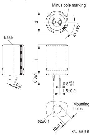
Snap-in terminals, length (6.3  $\pm$ 1) mm. Also available in a shorter version with a length of (4.5 -1) mm. Safety vent on the base.
