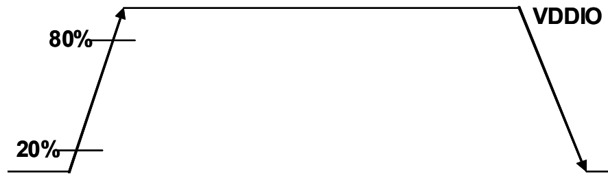
Figure 4. Output Pad Transition Waveform
