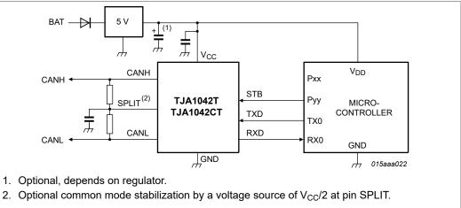
Figure 7. Typical TJA1042 application with a 5 V microcontroller (non-V<sub>IO</sub> variants)
