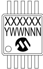
10-Lead MSOP (3x3 mm)
