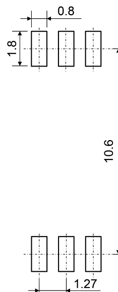
Fig. 15.2 Lead Forming Option (LF4)
