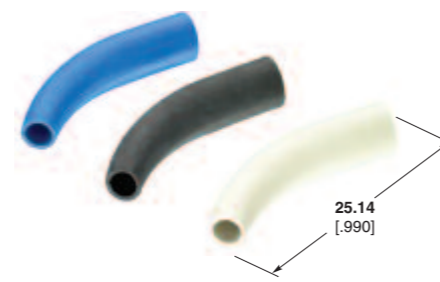
50 Degree Angle Boot for 1.6 to 2.4 mm Cable
