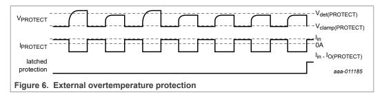
An internal clamp of 4.1 V (typical) protects this pin from excessive voltages.
