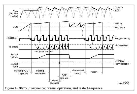
When the voltage on pin VCC drops to below the  $V_{th(UVLO)}$  level during normal operation, the controller stops switching. The TEA1833TS waits for the rectified mains to charge the VCC pin to  $V_{startup}$  using resistor R1.
