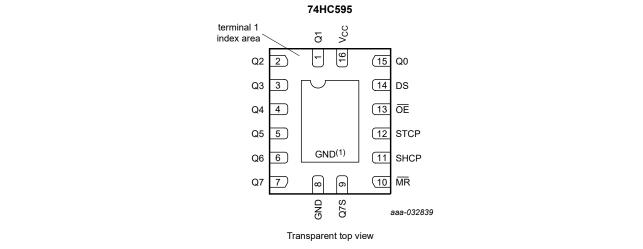
(1) This is not a ground pin. There is no electrical or mechanical requirement to solder the pad. In case soldered, the solder land should remain floating or connected to GND.
