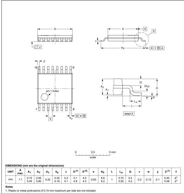
2. Plastic interlead protrusions of 0.25 mm maximum per side are not included.
