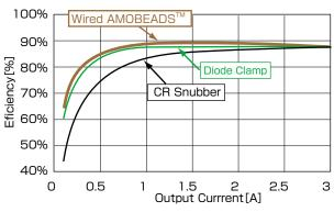
Power Supply Efficiency (Vin:DC140V, Vo:24V)
