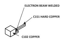
Figure 6 - Stress-relief Pin (SP Style)
