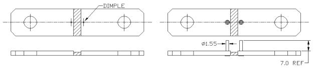
Figure 5 - Pressed Pin (PP Style)
