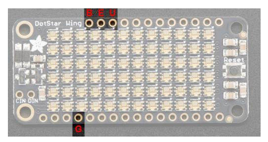
The Battery and Usb power pins are used to power the many DotStars. There's a lot of pixels and you can't really run them from the 3.3V regulator. Two 1A Schottkey diodes will automatically select whichever voltage is higher. That means, if USB is plugged in, you'll get ~5V USB power. If the feather is running off of battery power, say a LiPoly battery, you'll get 3.7-4.2V power. While this is a little lower than spec, DotStars are only a little dimmer.
