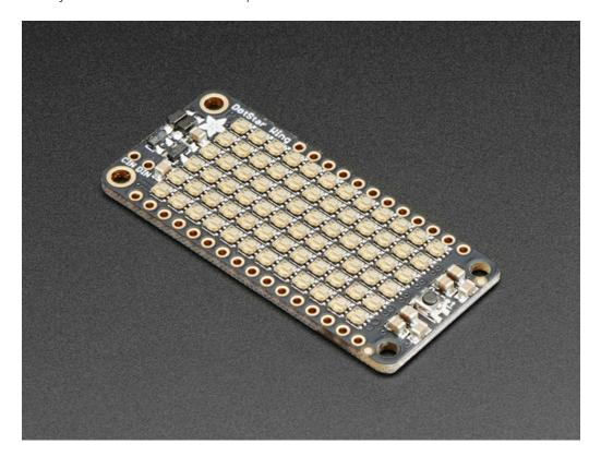
Put on your sunglasses before staring into these 72 configurable RGB LEDs, they are super bright! Arranged in a 6x12 matrix, each 2mm by 2mm sized RGB pixel is individually addressable. Only two pins are required to control all the LEDs. On the bottom we have jumpers for the Data and Clock lines so you can change them from the defaults. **Works with any/all of our Feathers!** You can cut the default jumper traces and use any pins you like
