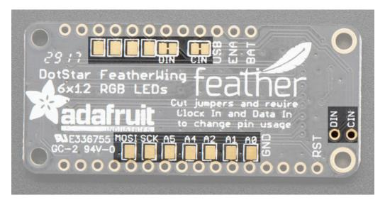
Note there is no logic level shifter for Clock and Data - we have not found that these chips require a level shifter, they work nicely at 3.3V logic even with 5V+ power
