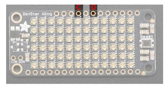
But - it's very easy to change the connections. On the bottom, you can cut the two jumper traces near those two pins, then solder wires from the **CIN** and **DIN** pins to the available square pads
