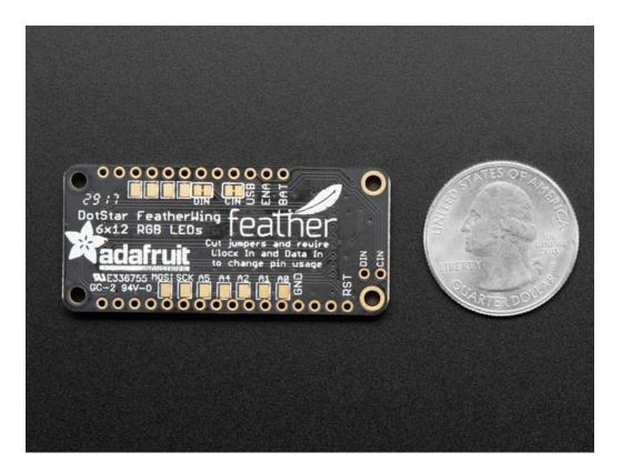
To make it easy to start, the LEDs are by default powered from *either* the USB power line or Battery power line, whichever is higher. Two Schottky diodes are used to switch between the two. This power arrangement is able to handle 1 Amp of constant current draw and maybe 2A peak, so not a good way to make a flashlight. It's better for colorful effects. A power MOSFET is set up and connected to the ENABLE pin on the Feather so that when the Feather is disabled, the wing will also cut power.
