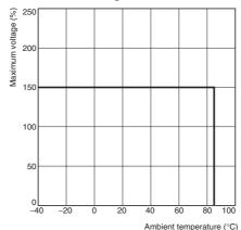
Ambient temperature (°C) "Maximum voltage" is the maximum voltage that can be applied to the Relay coil.
