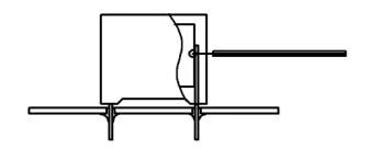
Temperature monitored inside the capacitor.
