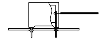
Temperature monitored inside the capacitor.
