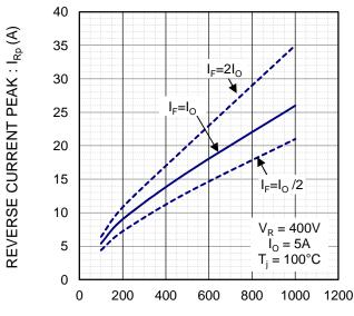
RATE OF CHANGE OF CURRENT :  $-di/dt(A/\mu s)$   $di/dt-I_{RD}$  CHARACTERISTICS
