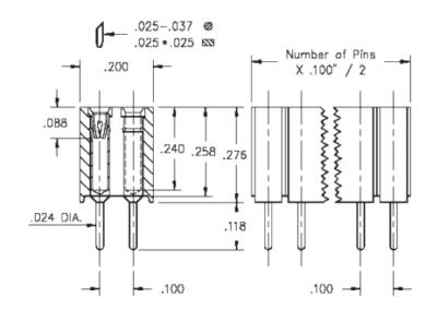
**Description:** Interconnect Socket Standard Solder Tail Socket Accepts .025" - .037" (0,635 - 0,94 mm)dia leads Double Row
