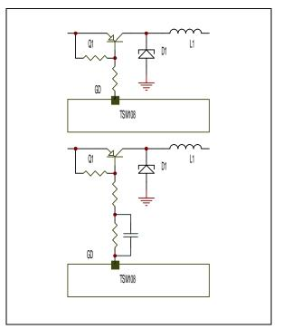
The most immediate way to choose between a P-channel MOSFET or a PNP transistor is to consider the ratio between the output power of the application and the expected components price: the lower the power, the more suitable the PNP transistor is; the higher the power, the more suitable the P-channel MOSFET is. As an example, for a DC/DC adaptor built for 12V/6V, the recommended limit to choose between P-channel Mosfet and PNP transistor is around 200mA.
