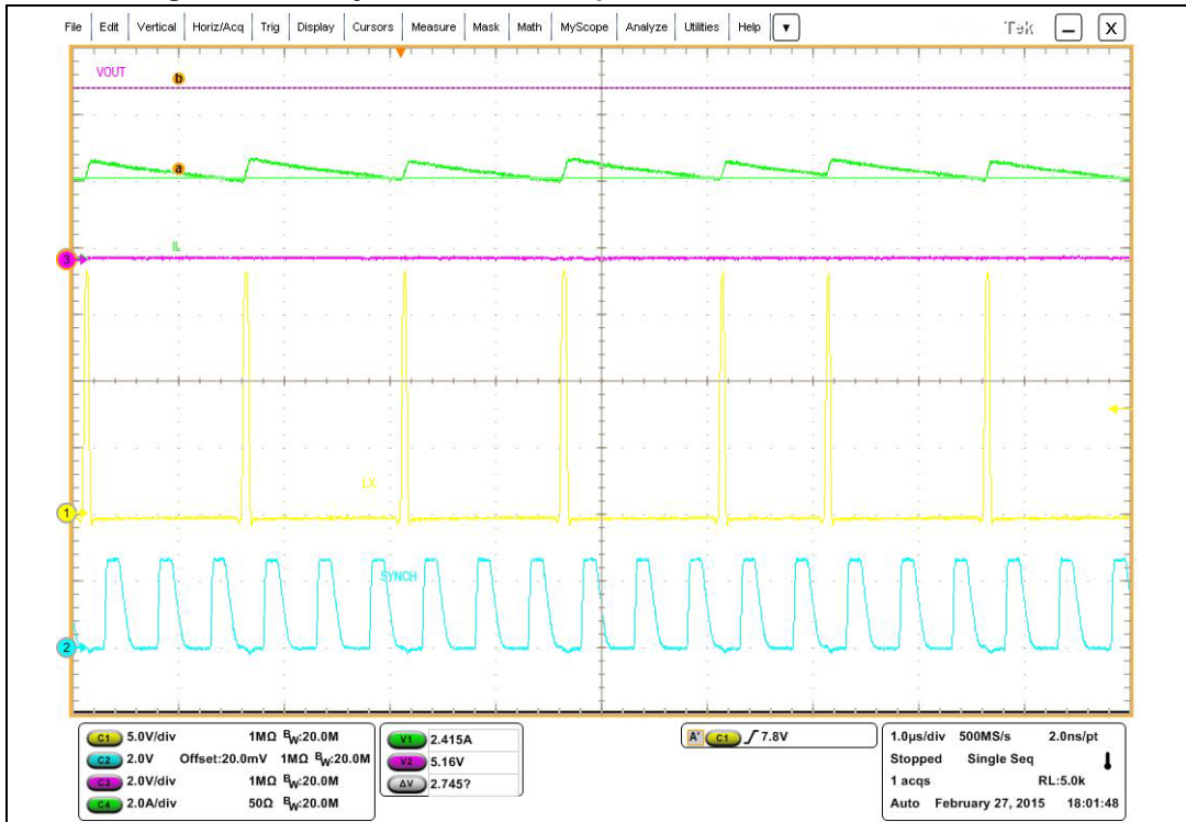
Figure 23. Valley current sense operation in overcurrent condition
