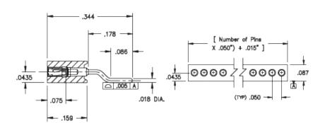
**Description:** Interconnect Socket Horizontal Mount Socket Accepts .015"- .020" (0,38 - 0,508 mm) dia leads Single Row Surface Mount **Plating Code:** 11 Shell Plating: 10 µ" Gold over 100 µ" Nickel **Inner Contact Plating:**
