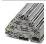
Motor terminal block, four-level, with PE foot, connection method: spring-cage connection, cross section: 0.08 mm² - 4 mm², AWG: 28 - 12, width: 5.2 mm, color: gray, mounting type: NS 35/7,5, NS 35/15
