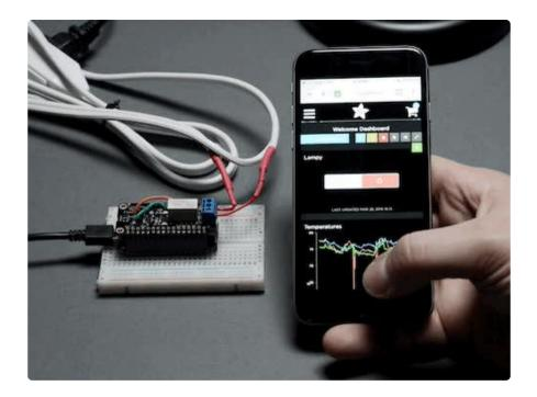
The are two 'flavors' of these FeatherWings, the first is the simple Non-Latching relay. This Wing has a single Set pin. Normally, the COM pin is connected mechanically to the NC pin and the NO pin is disconnected.
