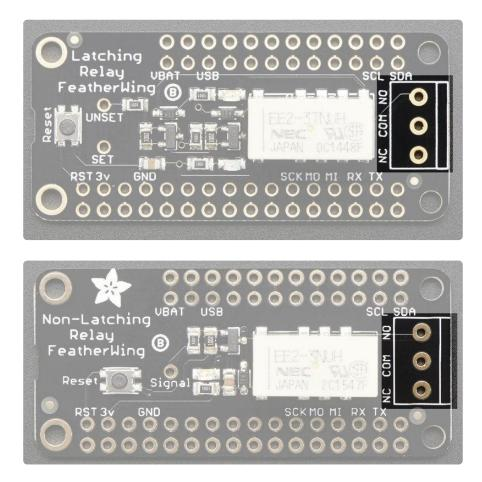
Both Wings have the same output, a 3-pin 3.5mm terminal block. The COM pin is what you should connect the signal you're planning to switch. If the relay is unset, the NC pin (Normally Connected) is mechanically connected to COM. NO (Normally Open) is mechanically disconnected.
