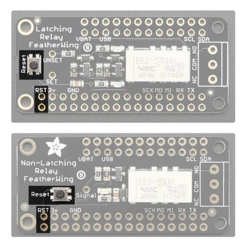
There is a Reset button on both Wings, this is connected to the RST pin and will short it to ground. It is not connected to the relay at all, its handy for restarting your Feather
