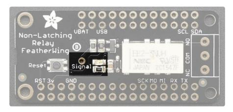
The plain relay uses a single pin for control. When the signal pin is floating or pulled low, the relay is 'open' or unset. When the signal pin is pulled high, the relay switches closed/set. A red LED next to the pin will let you know that the signal is high. You will need to solder a wire from this pin to whatever control pin you like using a wire
