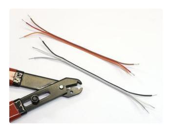
Separate the wires by about 1 inch at both ends, strip away a little insulation and give the wires a twist to prevent fraying.
