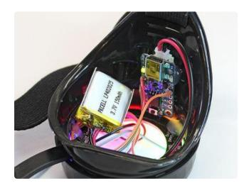
Power on the goggles by connecting the battery.
