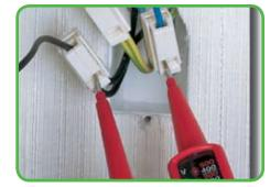
Testing through separate test slot
