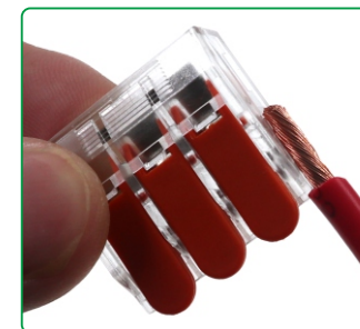
1) Strip the wire length 10-12mm
