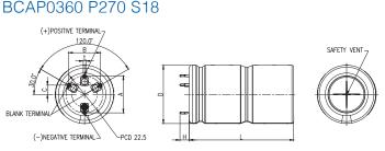
RECOMMENDED PCB PATTERN HOLE SIZE : 2.0(±0.1)mm
