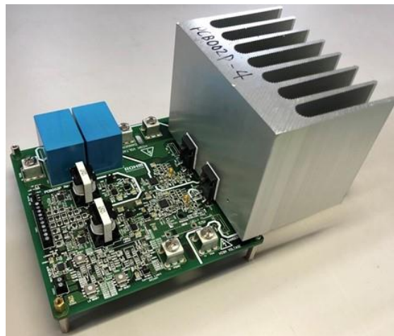
Figure 21. Heatsink Installation Example
