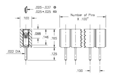
Interconnect Socket Standard Solder Tail Socket Accepts .025"- .037" (0,635 - 0,94 mm)dia leads Single Row Through Hole Plating Code: 41 Shell Plating: 200 µ" Tin (matte finish) over 100 µ" Nickel Inner Contact Plating:
