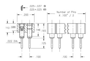
**Description:** Interconnect Socket Standard Solder Tail Socket Accepts .025" - .037" (0,635 - 0,94 mm)dia leads Double Row Through Hole Plating Code:
