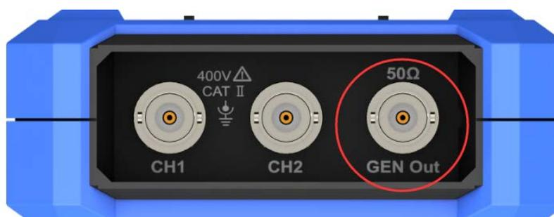
Figure 5-1 : Generator Output Ports
