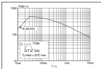
Fig.2. Maximum permissible non-repetitive peak on-state current  $I_{TSM}$ , versus pulse width  $t_p$ , for sinusoidal currents,  $\dot{t}_p \leq 10$ ms.
