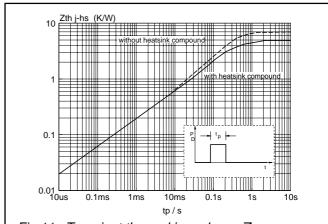
Fig.11. Transient thermal impedance  $Z_{th j-hs}$ , versus pulse width  $t_p$ .
