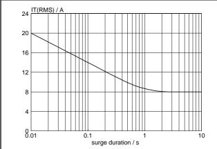
Fig.5. Maximum permissible repetitive rms on-state current  $I_{T(RMS)}$ , versus surge duration, for sinusoidal currents, f = 50 Hz;  $T_{hs} \le 90$  °C.
