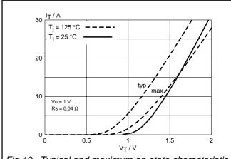
Fig. 10. Typical and maximum on-state characteristic.
