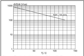
Fig. 12. Typical, critical rate of rise of off-state voltage,  $dV_D/dt$  versus junction temperature  $T_{j\cdot}$
