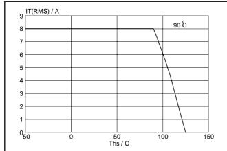
Fig.3. Maximum permissible rms current  $I_{T(RMS)}$ , versus mounting base temperature  $T_{hs}$ .
