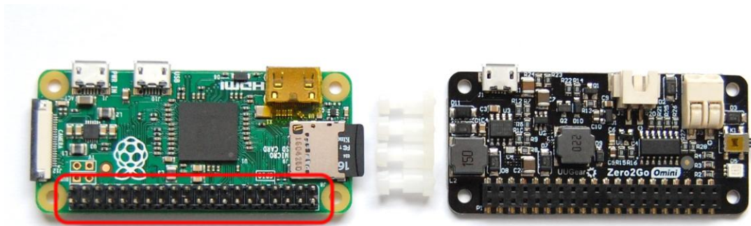
Header must be soldered on Raspberry Pi Zero (W)
