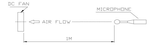
NOISE IS MEASURED AT RATED VOLTAGE IN FREE AIR IN SEMI-ANECHOIC CHAMBER WITH B & K SOUND LEVEL METER WITH MICROPHONE AT A DISTANCE OF 1M FROM THE FAN INTAKE.
