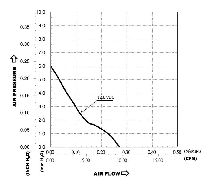
\*TEST CONDITION: INPUT VOLTAGE-----OPERATION VOLTAGE
