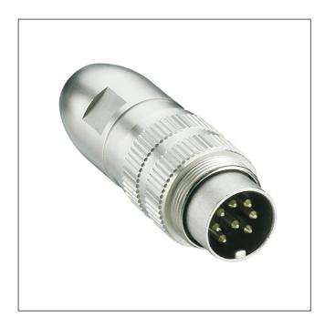
Plug acc. to AISG specification and IEC 61076-2-106, IP68, with threaded joint and solder terminals, shielded at 360°
