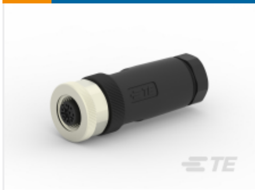
TE Part #T4110002081-000 M12,FEMALE,STRAIGHT,A CODE,8P, PG9,GOLD
