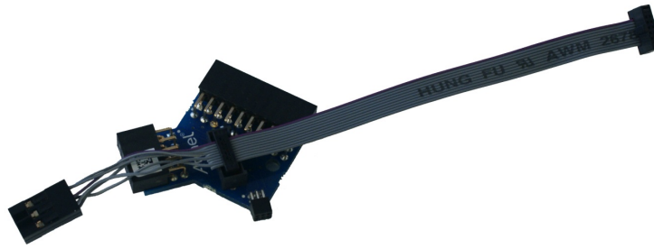
Figure 2-10. Atmel-ICE AVR Probe Connection
