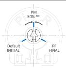
Wiper positioning on initial position is standard. Special delivery positions available on request.
