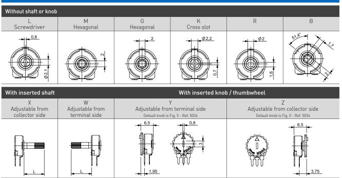
Default delivery is at initial position. Wipers are shown positioned at 50% for the picture.
