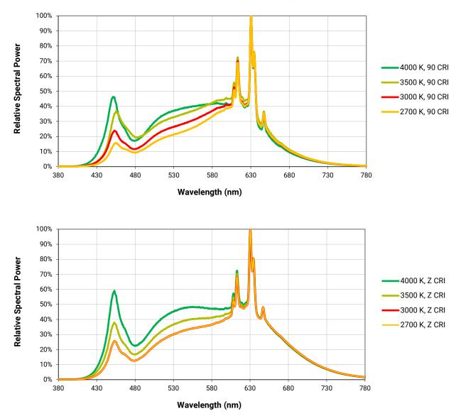
The following graphs are the result of a series of pulsed measurements at 990 mA and  $T_1$  = 85 °C.
