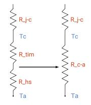
As the figure at right shows, the R\_c-a value is the sum of the thermal resistance of the TIM (R\_tim) plus the thermal resistance of the heat sink (R\_hs).
