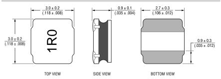
Note: Top and side view dimensions do not include termination. For maximum overall dimensions including termination, add 0.1 mm.
