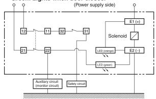
2. Orange: Lights when the solenoid turns ON. Green: Lights when power turns ON.
