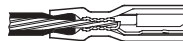
Cross section of DiscoGrip ™ crimp showing insulation crimp of the wire insulation.
