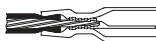
Cross section of DiscoGrip ™ crimp showing insulation crimp of the wire insulation.
