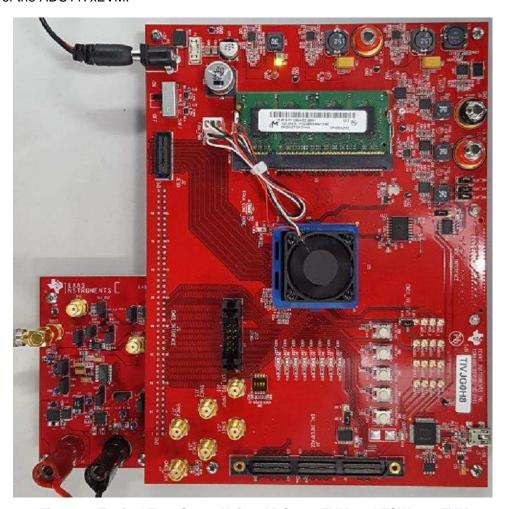
Figure 3. Typical Test Setup Using ADC117xEVM and TSW1400EVM
