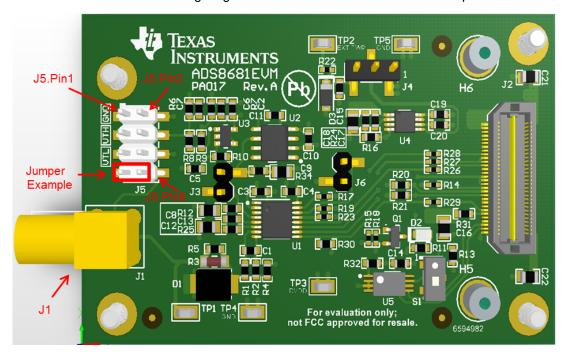
Figure 3. Connectors and Jumpers for Input
