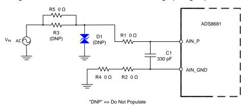
Figure 2. Schematic of Input Signal Path
