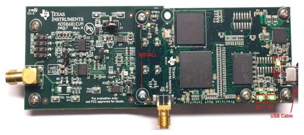
Figure 9. EVM-PDK Hardware Setup and LED Indicators
