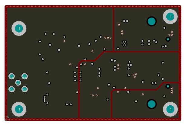
Figure 19. ADS8681EVM PCB Layer 3 - Power Planes
