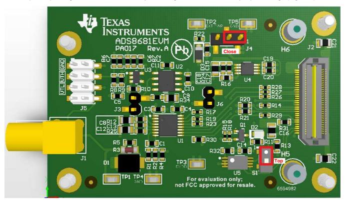
Figure 5. Default Settings for Jumper and Switch
