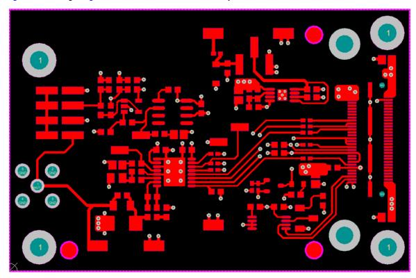
Figure 17. ADS8681EVM PCB Layer 1 – Top Layer
