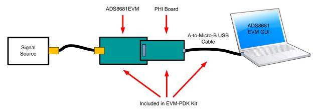
Figure 1. System Connection for Evaluation
