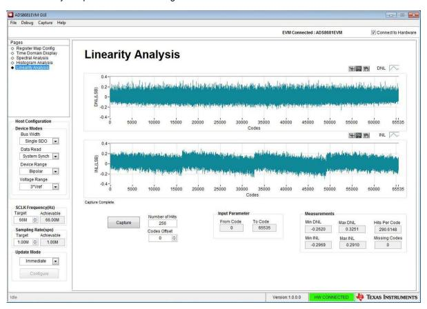
Figure 16. Linearity Analysis Tool
