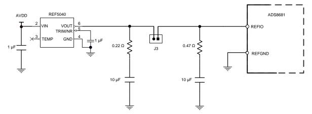
Figure 4. On-Board Reference Signal Path
