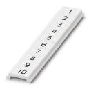
Zack Marker strip, flat, Strip, white, labeled, Printed vertically: consecutive numbers 1 ... 10, 11 ... 20, etc. up to 91 ... 100, mounting type: snapped, for terminal block width: 3.5 mm, lettering field size: 5.15 x 3.5 mm, Number of individual labels: 10
