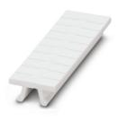
Zack marker strip, Strip, white, unlabeled, can be labeled with: PLOTMARK, CMS-P1-PLOTTER, mounting type: snapped, for terminal block width: 3.5 mm, lettering field size: 3.5 x 10.5 mm, Number of individual labels: 10
