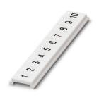
Zack Marker strip, flat, Strip, white, labeled, printed horizontally: consecutive numbers 1  $\dots$  10, 11  $\dots$  20, etc. up to 91  $\dots$  100, mounting type: snapped, for terminal block width: 3.5 mm, lettering field size: 5.15 x 3.5 mm, Number of individual labels: 10
