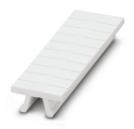
Zack marker strip, can be ordered: Strip, white, labeled according to customer specifications, mounting type: snap into tall marker groove, for terminal block width: 3.5 mm, lettering field size:  $3.5 \times 10.5 \text{ mm}$ , Number of individual labels:  $10 \times 10^{-5}$
