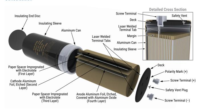
Screw Terminal Aluminum Electrolytic Capacitors - ALS60/61 Series, +85°C
